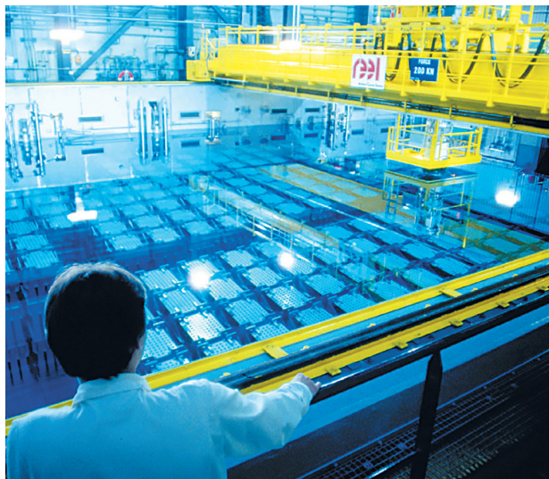
Spent fuel storage pool at the Orano reprocessing plant in La Hague
