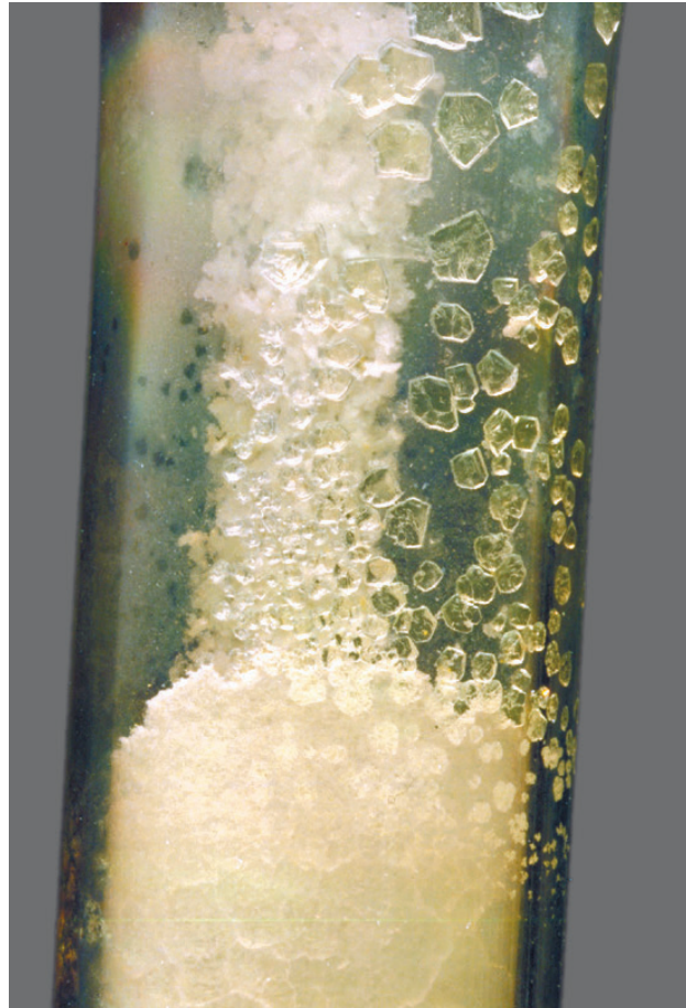
Uranium hexafluoride crystals
